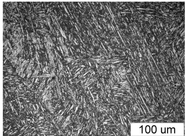
Fig. 6. Microstructure of welded joint of VM12SHC steel
