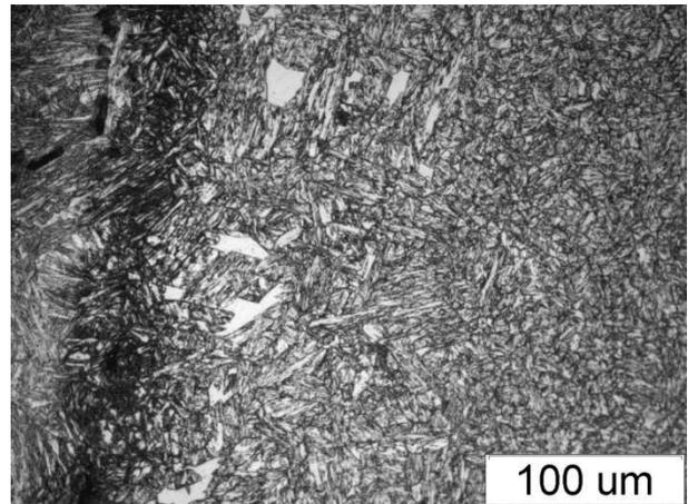
Fig. 4. HAZ microstructure of welded joint of HR3C steel
