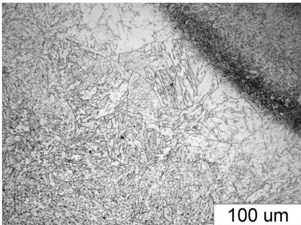
Fig. 5. BM microstructure of welded joint of 10CrMo910 steel
