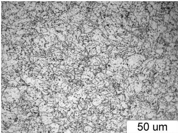
Fig. 3. HAZ microstructure of welded joint of HR3C steel
