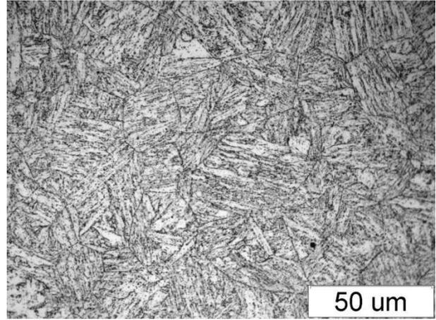
Fig. 2. BM microstructure of welded joint of VM12SHC steel
