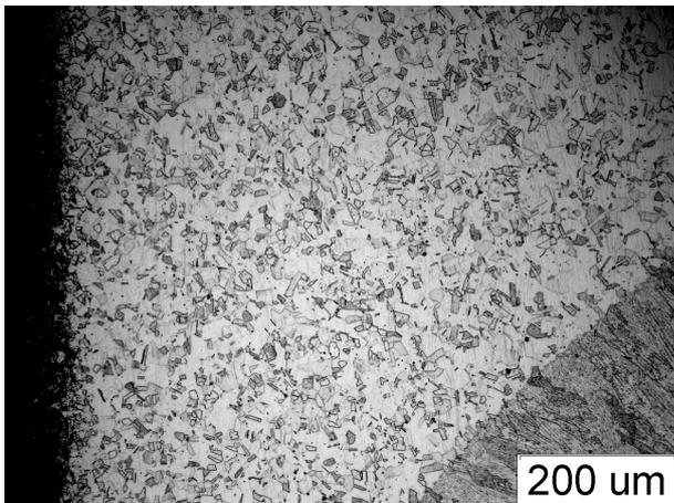
Fig. 3. HAZ microstructure of the 3R12 pipe
