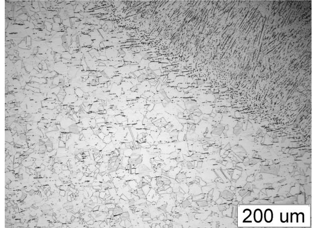
Fig. 2. HAZ microstructure of the flat bar made of X6CrNi18-10 steel
