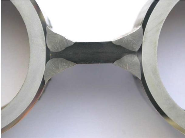
Fig. 1. Macrostructure of the welded joint
