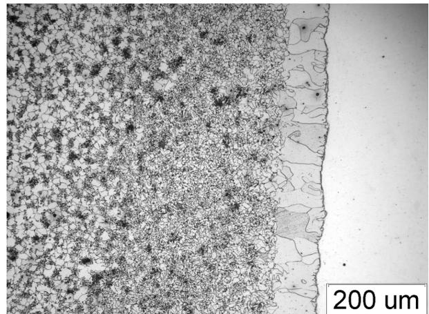
Fig. 4. HAZ microstructure of the 4L7 pipe
