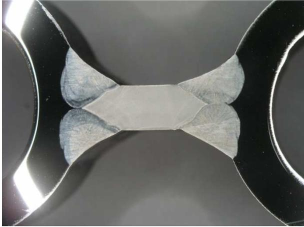
Fig. 1. Macrostructure of welded joint of VM12SHC steel
