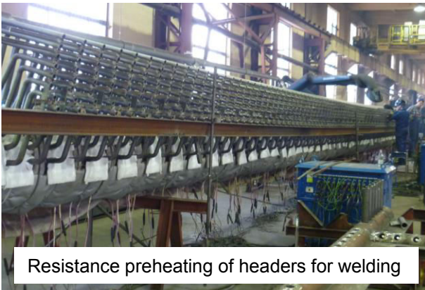
Resistance PWHT of T91 coils butt joints
