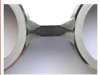
Fig. 1. Macrostructure of the welded joint
