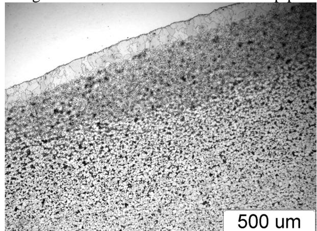
Fig. 6. Microstructure of the pipe in the area of the sample rupture
