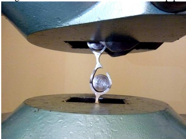
Fig. 5. View of the sample after rupture in the wall of the pipe
